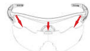
The system of interchangeable lenses called Easy-Change is one of the basic technologies of our sport glasses. Every sport glasses model has different way of fitting and removing the lenses. The shape of the lenses and the frame interact differently. Easy-Change technology enables you to easily change out lenses to manage any light condition.
